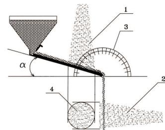
**Fig. 1.** Set-ups and geometries for a pre-sowing laser treatment of seeds: 1 – divergent laser beam geometry used when a constant seeds speed is chosen, 2 – divergent laser beam geometry used when seeds freely fall down with acceleration characteristic for the gravity, 3 – angle gauge, 4 – illuminated area where seeds are biostimulated with a laser beam,  $\alpha$  – angle of inclination of the trough.
