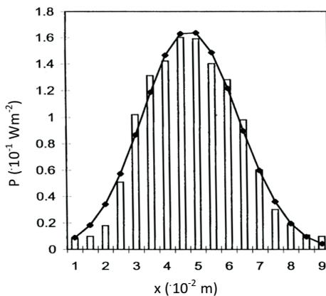
**Fig. 2.** Distribution of the surface power density of laser radiation fitted with a Gaussian function ( $\sigma = 1.56 \cdot 10^{-2} \text{ m}$ ,  $x_{\text{mean}} = 4.77 \cdot 10^{-2} \text{ m}$ ,  $P_{\text{max}} = 16.5 \cdot 10^{-2} \text{ W m}^{-2}$ ).
