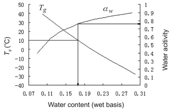
**Fig. 4.** Relationship between the water activity ( $\alpha_w$ ), water content and glass transition temperature ( $T_g$ ) of the heat pump dried squid stored at 10°C.
