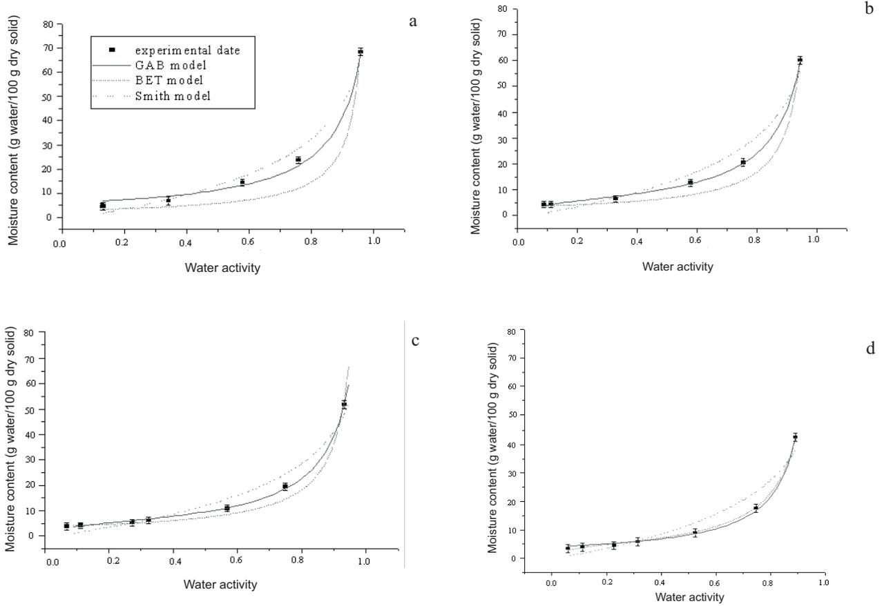
**Fig. 2.** Experimental data for heat pump-dried squid and predicted sorption isotherms using three model equations at different temperatures: a – 10, b – 20, c – 30, and d – 40°C.
