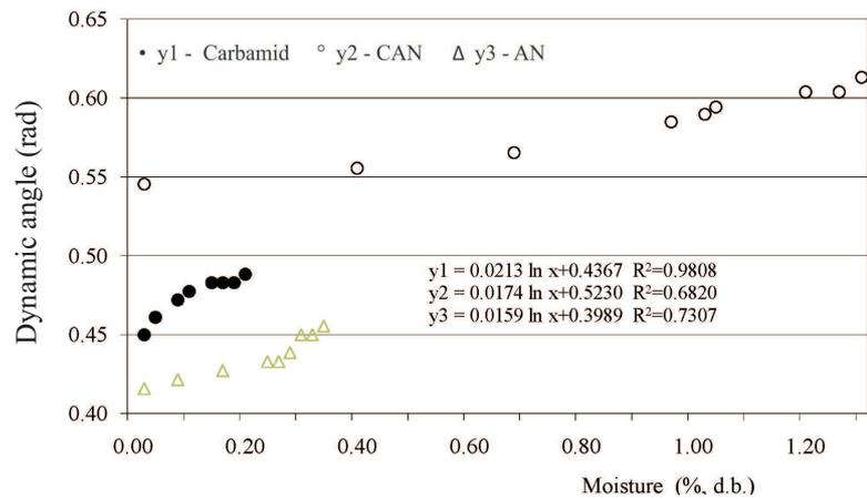
Fig. 3. Dynamic angle of repose depending on humidity.
