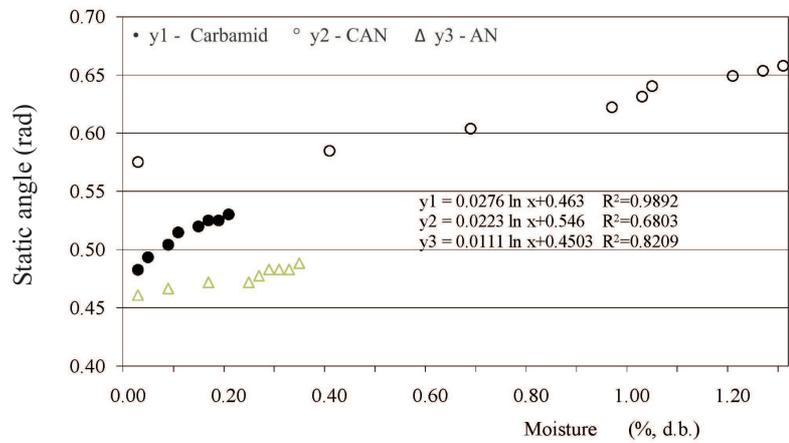
Fig. 2. Static angle of repose depending on humidity.
