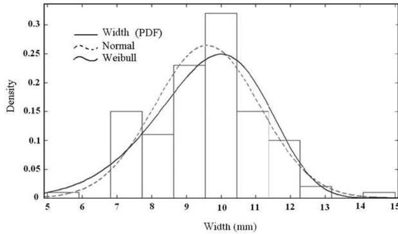
**Fig. 4.** Histogram of raisin berries probability density function for width dimension by comparing its fitting behaviour between normal and Weibull distributions (at the %16 (d.b) moisture content).
