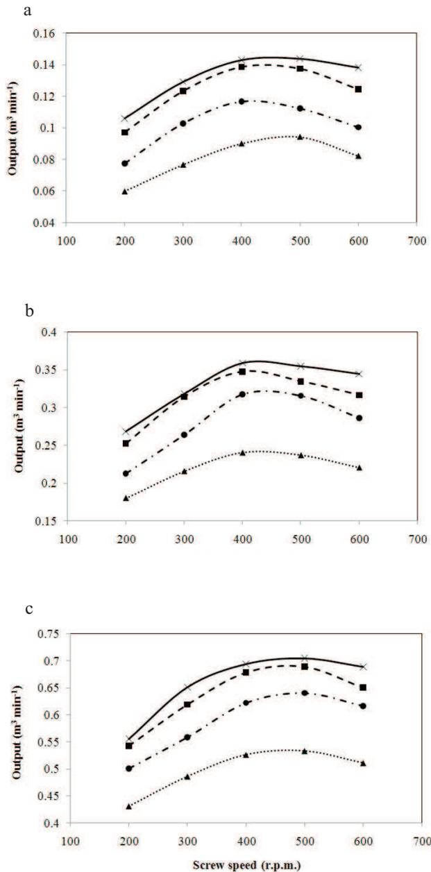
**Fig. 1.** Effect of screw rotational speed and conveying inclination on the volumetric output for: a – 15.5, b – 20, and c – 25 cm screw augers; × horizontal conveying, ■ 10, ● 20, and ▲ 30°.
