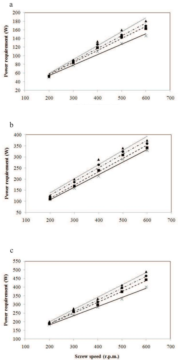
**Fig. 3.** Effect of screw rotational speed and conveying inclination on the power requirements for: a – 15.5, b – 20, and c – 25 cm screw augers; × horizontal conveying, ■ 10, ● 20, and ▲ 30°.
