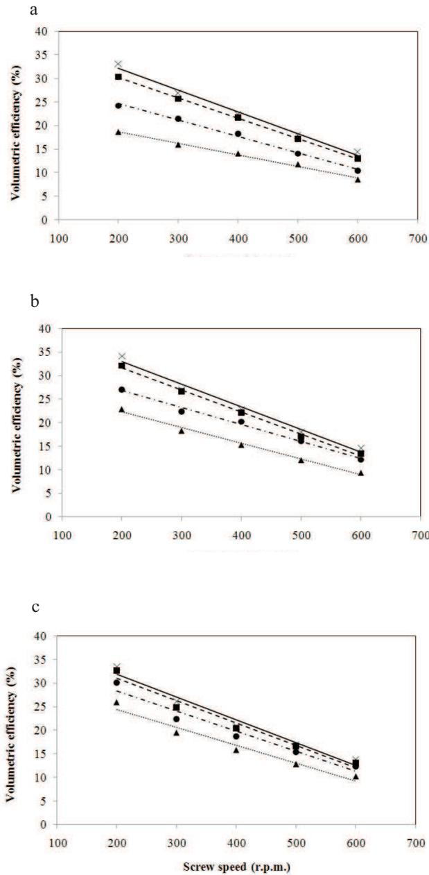
**Fig. 2.** Effect of screw rotational speed and conveying inclination on the volumetric efficiency for: a – 15.5, b – 20, and c – 25 cm screw augers; × horizontal conveying, ■ 10, ● 20, and ▲ 30°.
