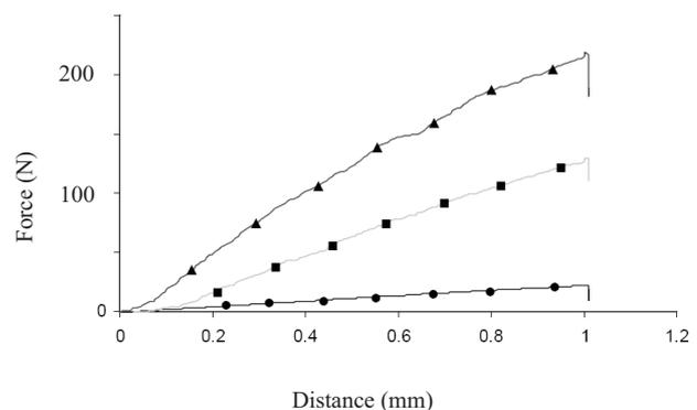
Fig. 2. Typical force-deformation plot which resulted from tension loading of a specimen: ▲ upper, ■ middle, and ● lower regions.
