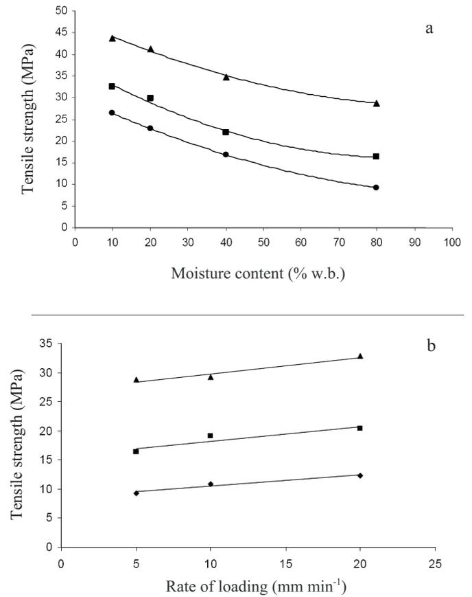
**Fig. 3.** Changes of tensile strength with: a – moisture content, b – rate of loading according to the regions: ▲ lower; ■ middle, and ● upper.
