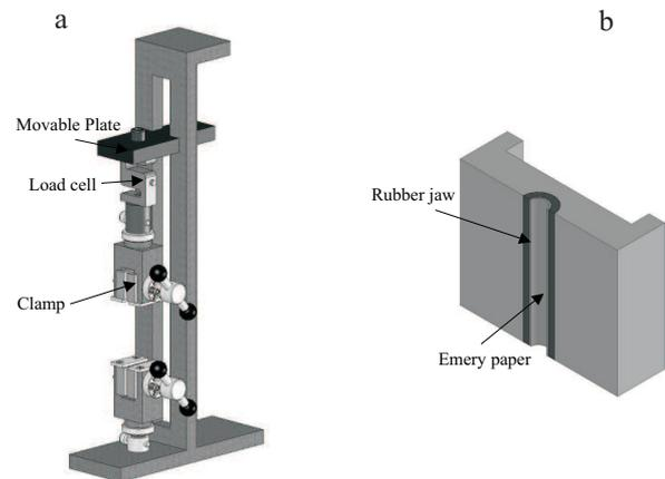
Fig. 1. Apparatus for the measurement of tensile strength: a – schematic of apparatus, b – clamp.
