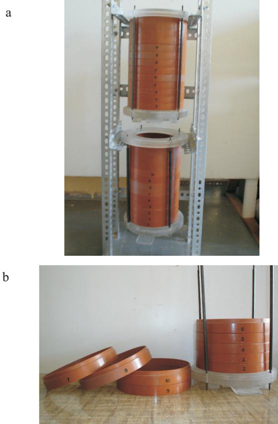
Fig. 2. Flow mixer: a – view of the whole equipment, b – modular design of the silo (own study).
