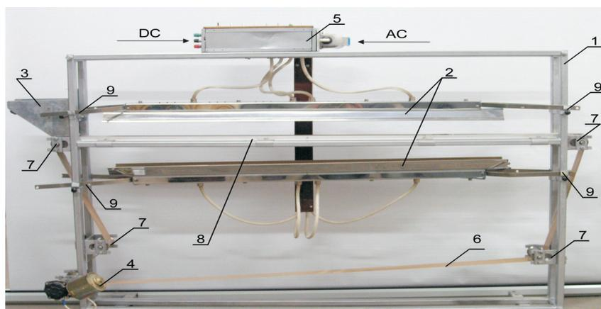
**Fig. 1.** Laboratory device for infra-red radiation treatment of pea seeds: 1 – frame, 2 – infra-red radiators, 3 – feeding tank, 4 – electric motor, 5 – control unit, 6 – conveyor belt, 7 – rollers, 8 – heating zone, 9 – adjustment of heads position.
