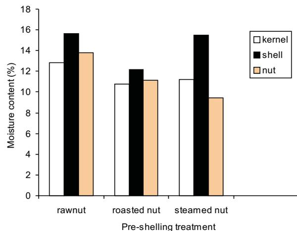
**Fig. 2.** Effects of pre-shelling treatment on the moisture content of structural components of cashew nut.
