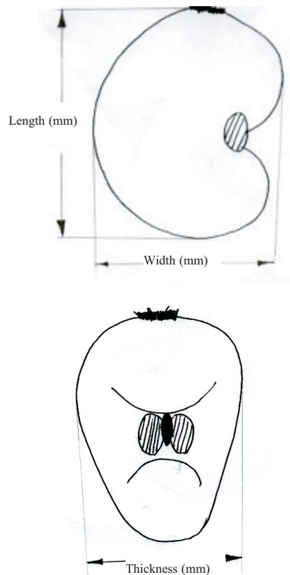
Fig. 1. Schematic diagram showing the characteristic dimensions of cashew nut.
