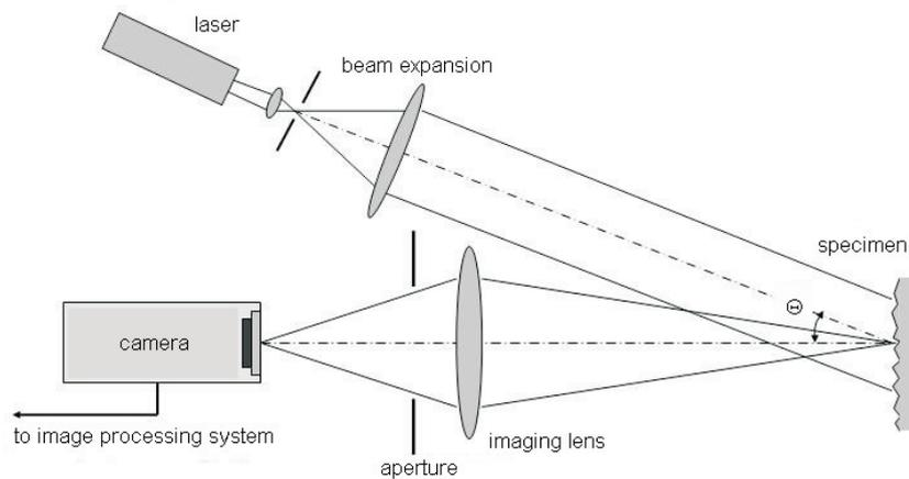
**Fig. 2.** Experimental setup for Digital Speckle Correlation system.
