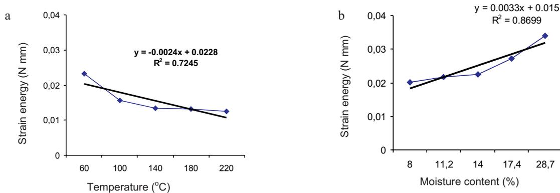
Fig. 5. Effect of temperature (a) and moisture content (b) on strain energy.
