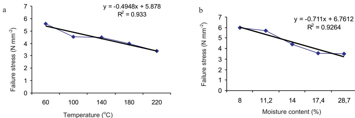
Fig. 4. Effect of temperature (a) and moisture content (b) on failure stress.
