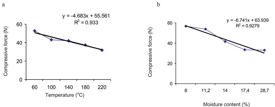
**Fig. 2.** Effect of temperature (a) and moisture content (b) on compressive force.
