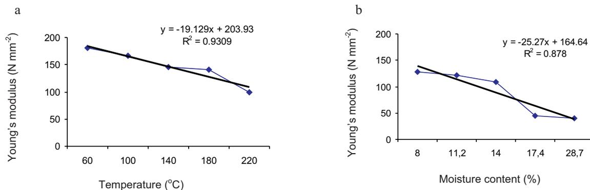
Fig. 6. Effect of temperature (a) and moisture content (b) on Young's modulus.
