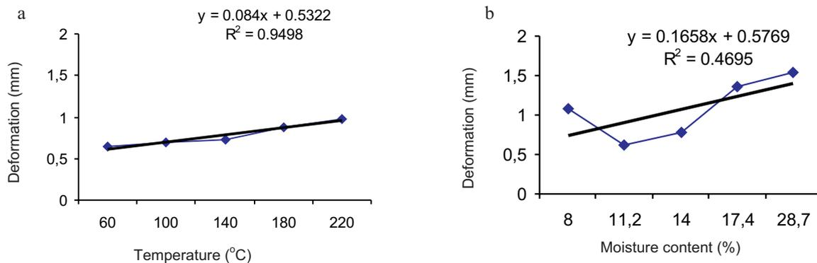
**Fig. 3.** Effect of temperature (a) and moisture content (b) on deformation.
