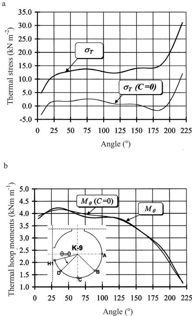
Fig. 8. Selected diagrams for outer arch of silo bin K-9 at the level of 5.5 m: a) uniform thermal hoop stresses in concrete, b) thermal hoop moments.
