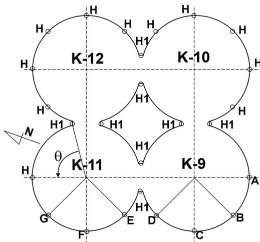
**Fig. 2.** Location of temperature test points on the surface of grain silo battery perimeter.
