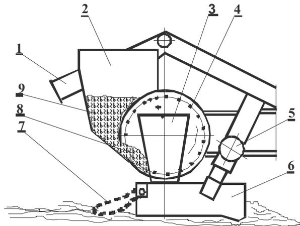
**Fig. 1.** Construction schematic and principle of operation of S071/B KRUK seeder sowing system: 1 – frame, 2 – reservoir, 3 – seeding trough, 4 – seeding disk with spoons, 5 – lock mechanism of furrow opener position, 6 – furrow opener, 7 – firmer, 8 – seed reservoir outlet, 9 – seeds.
