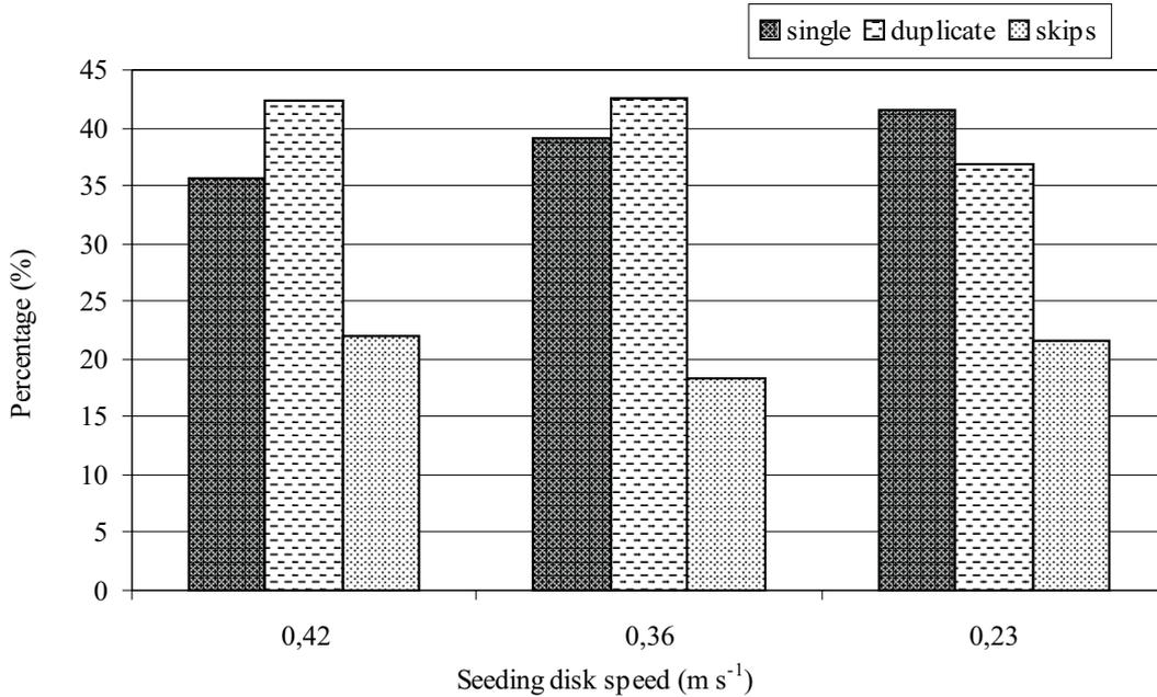
Fig. 2. Influence of peripheral speed of sowing disk of S071/B seeder on percentages of single, duplicate and skipped plants.
