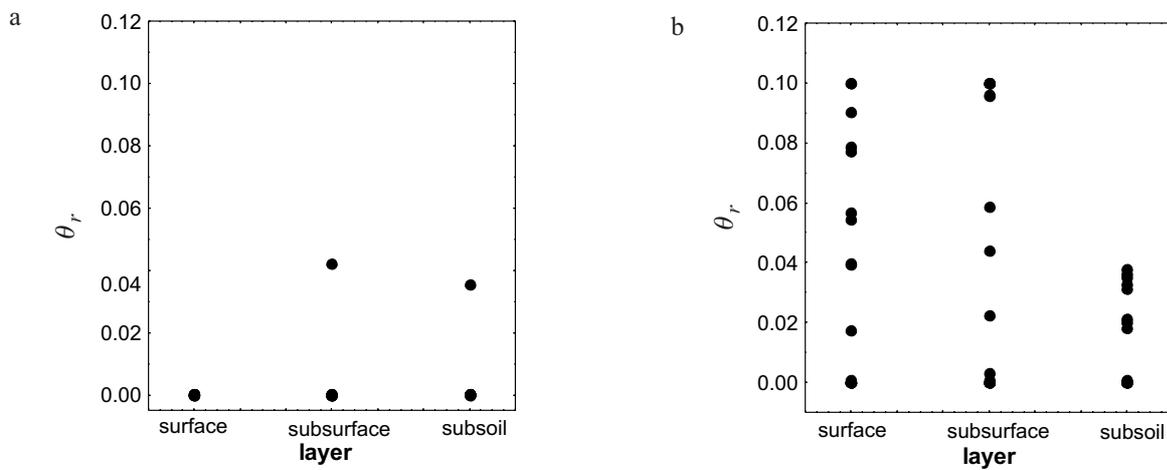
Fig. 6. Values of  $\theta_r$  for three investigated layers for: a) Phaeozems and b) Gleysols.
