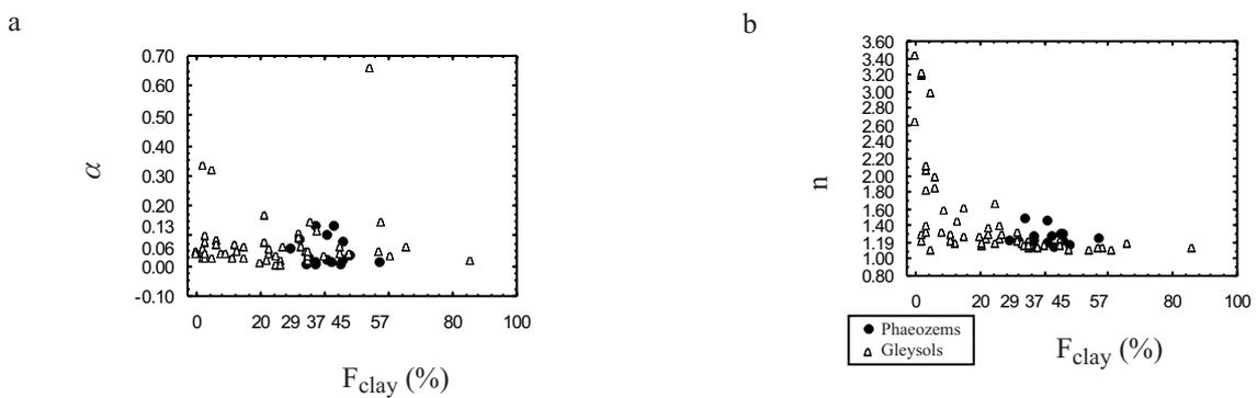
Fig. 9. Parameter versus clay content for: a)  $\alpha$  and b)  $n$ .
