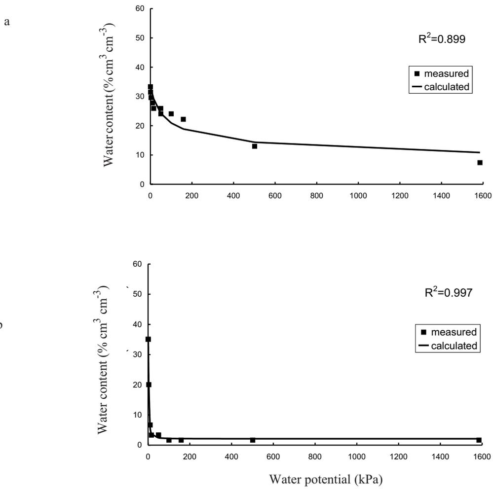
Fig. 2. Correlation between measured and calculated values of water retention content for Gleysols: a) the worst and b) the best.
