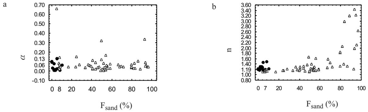
Fig. 7. Parameter versus sand content for: a)  $\alpha$  and b)  $n$ .
