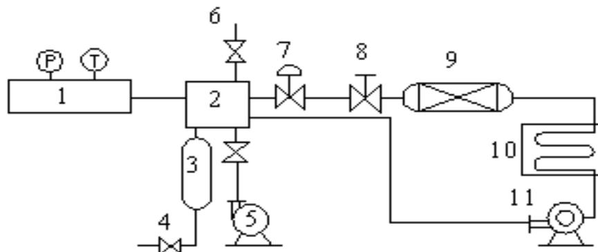
**Fig. 1.** Schemate of the vacuum cooler: 1 – vacuum chamber, 2 – steam condenser, 3 – condensing unit, 4 – draining valve, 5 – vacuum pump, 6 – vent valve, 7 – expansion valve, 8 – solenoid electric valve, 9 – filter dryer, 10 – condenser, 11 – compressor.
