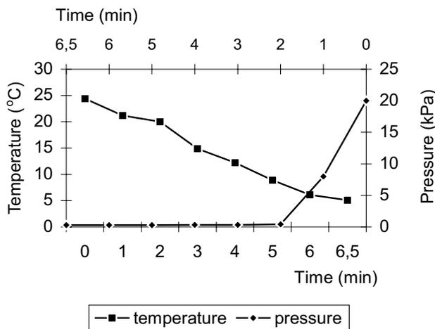
Fig. 2. Temperature and pressure change during vacuum cooling.
