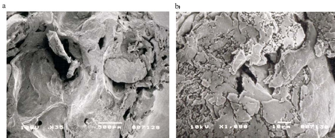
**Fig. 13.** The influence of moisture content on the macro- (a) and microstructure (b) of the twin screw extrudate: 30% rate of oat bran, extrusion-cooker 2S 9/5, extrusion temperature 180°C, moisture content 33%, die diameter 3.2 mm.
