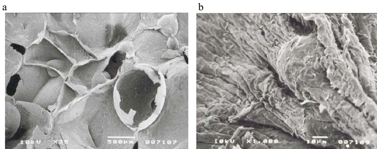
**Fig. 1.** Macro- (a) and microstructure (b) of the single screw extrudate: 9% rate of oat bran, extrusion-cooker S 45, extrusion temperature 120°C, moisture content 13.5%, die diameter 3 mm.
