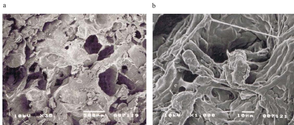
**Fig. 10.** The influence of extrusion temperature on the macro- (a) and microstructure (b) of the twin screw extrudate: 30% rate of oat bran, extrusion-cooker 2S 9/5, extrusion temperature 220°C, moisture content 24%, die diameter 3.2 mm.
