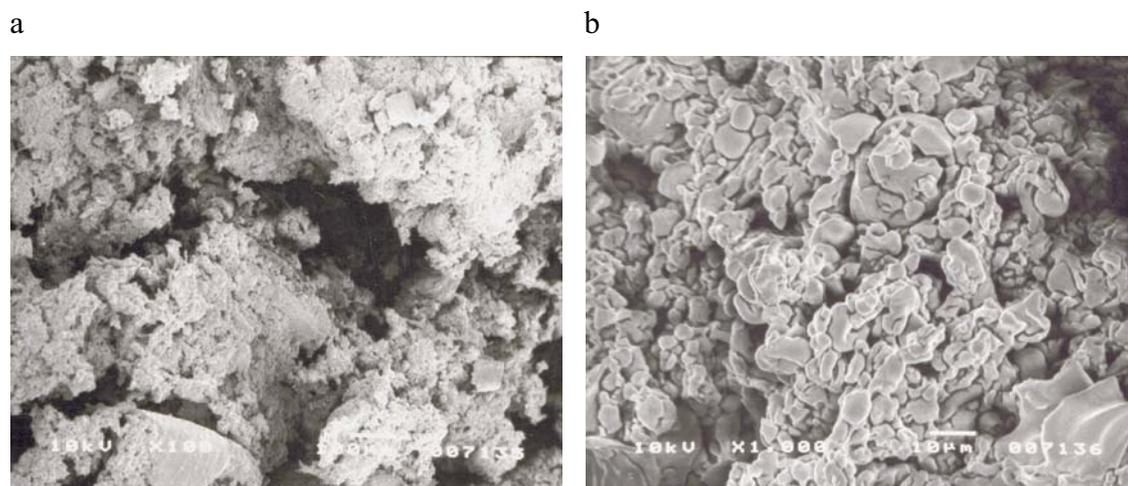
**Fig. 6.** The influence of oat bran rate on the macro- (a) and microstructure (b) of the twin screw extrudate: 80% rate of oat bran, extrusion-cooker 2S 9/5, extrusion temperature 180°C, moisture content 15%, die diameter 3.2 mm.
