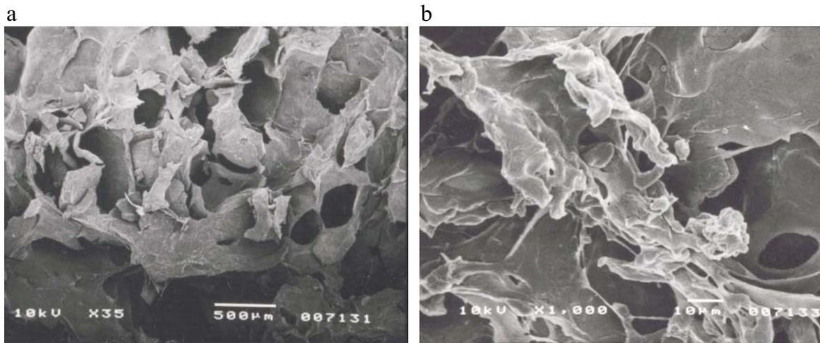
Fig. 4. The influence of oat bran rate on the macro- (a) and microstructure (b) of the twin screw extrudate: 20% rate of oat bran, extrusion-cooker 2S 9/5, extrusion temperature 180°C, moisture content 15%, die diameter 3.2 mm.
