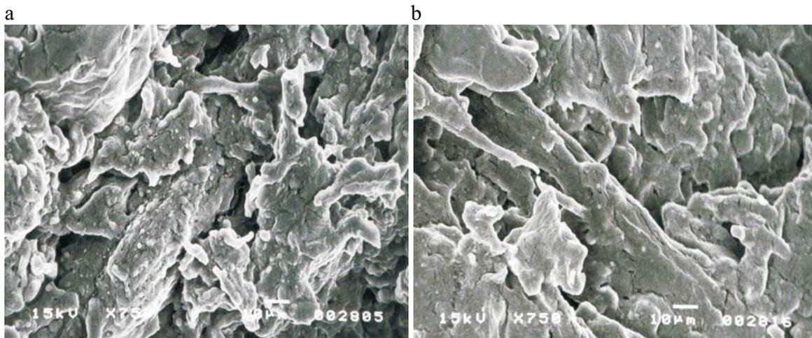
**Fig. 16.** Microstructure of the lupine extrudate: extrusion-cooker S 45; a) extrusion temperature 220°C, moisture content 15%, die diameter 3 mm; b) extrusion temperature 220°C, moisture content 30%, die diameter 3 mm.
