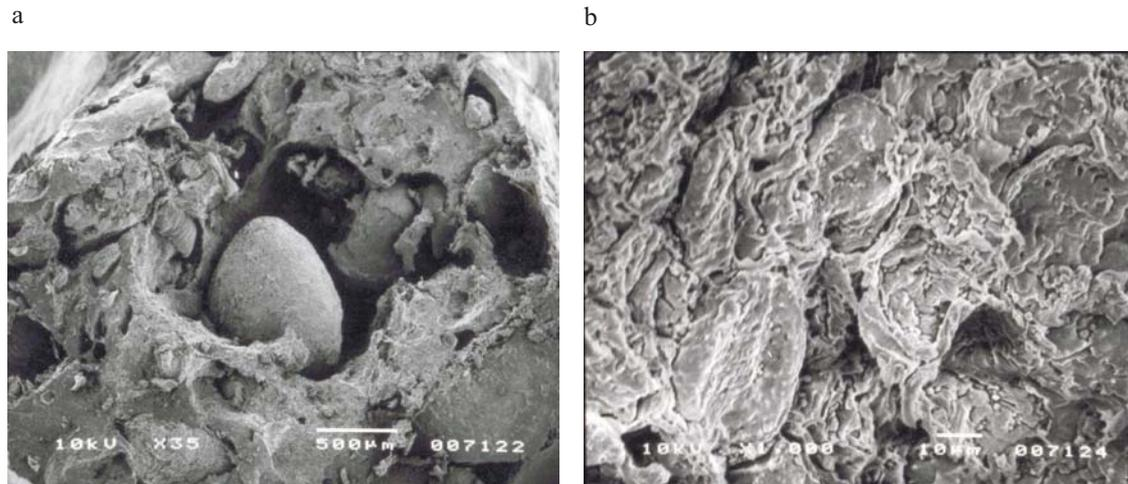
**Fig. 9.** The influence of extrusion temperature on the macro- (a) and microstructure (b) of the twin screw extrudate: 30% rate of oat bran, extrusion-cooker 2S 9/5, extrusion temperature 120°C, moisture content 24%, die diameter 3.2 mm.
