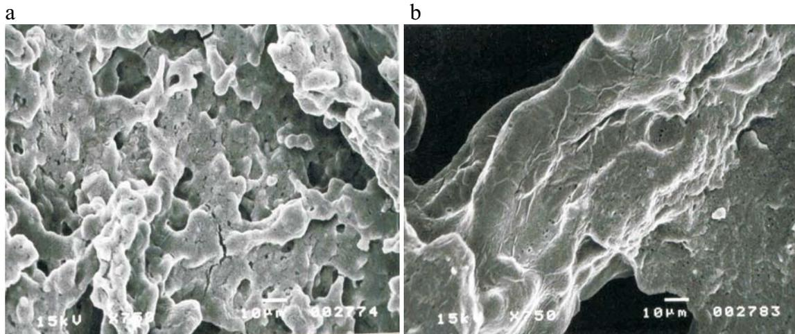
**Fig. 15.** Microstructure of the lupine extrudate: extrusion-cooker S 45; a) extrusion temperature 120°C, moisture content 15%, die diameter 3 mm; b) extrusion temperature 120°C, moisture content 30%, die diameter 3 mm.
