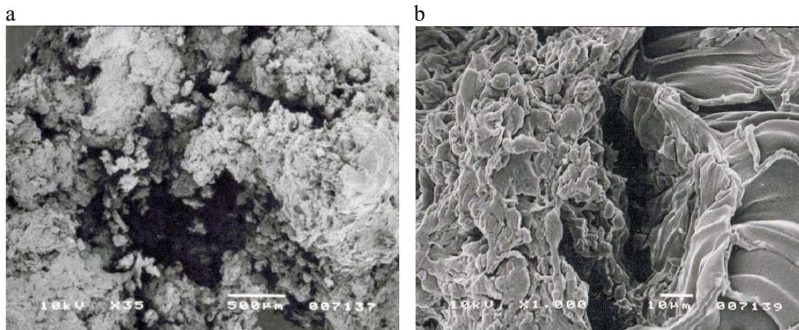
**Fig. 5.** The influence of oat bran rate on the macro-(a) and microstructure (b) of the twin screw extrudate: 40% rate of oat bran, extrusion-cooker 2S 9/5, extrusion temperature 180°C, moisture content 15%, die diameter 3.2 mm.
