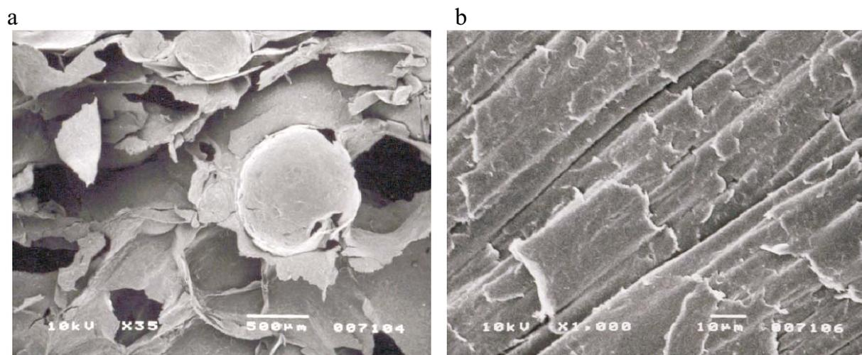
**Fig. 2.** Macro- (a) and microstructure (b) of the single screw extrudate: 9% rate of oat bran, extrusion-cooker S 45, extrusion temperature 180°C, moisture content 13.5%, die diameter 3 mm.
