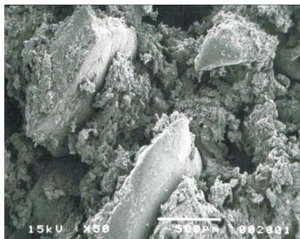
**Fig. 14.** Macrostructure of the lupine extrudate: extrusion-cooker S 45, extrusion temperature 180°C, moisture content 15%, die diameter 3 mm.
