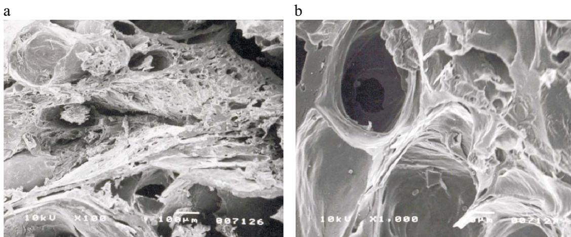
Fig. 12. The influence of moisture content on the macro- (a) and microstructure (b) of the twin screw extrudate: 30% rate of oat bran, extrusion-cooker 2S 9/5, extrusion temperature 180°C, moisture content 15%, die diameter 3.2 mm.
