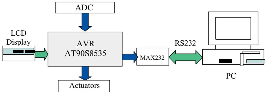
Fig. 2. Schematic of greenhouse control and monitoring system.
