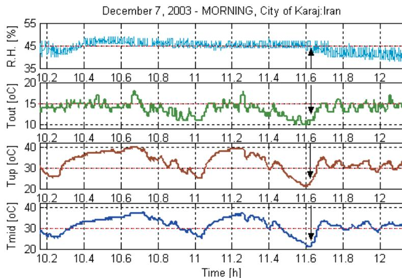
Fig. 4. Temperature and humidity variations inside and outside greenhouse.
