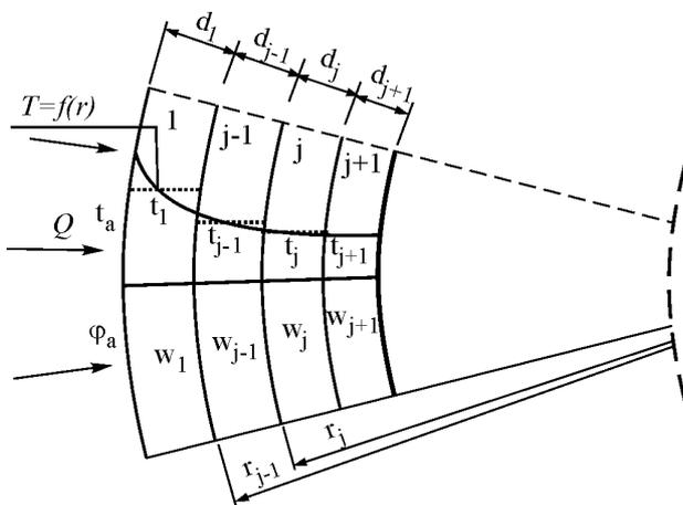
Fig. 2. Assumptions for the analysis of unsteady axi-symmetric heat flow coupled with moisture migration in cylindrical coordinates.
