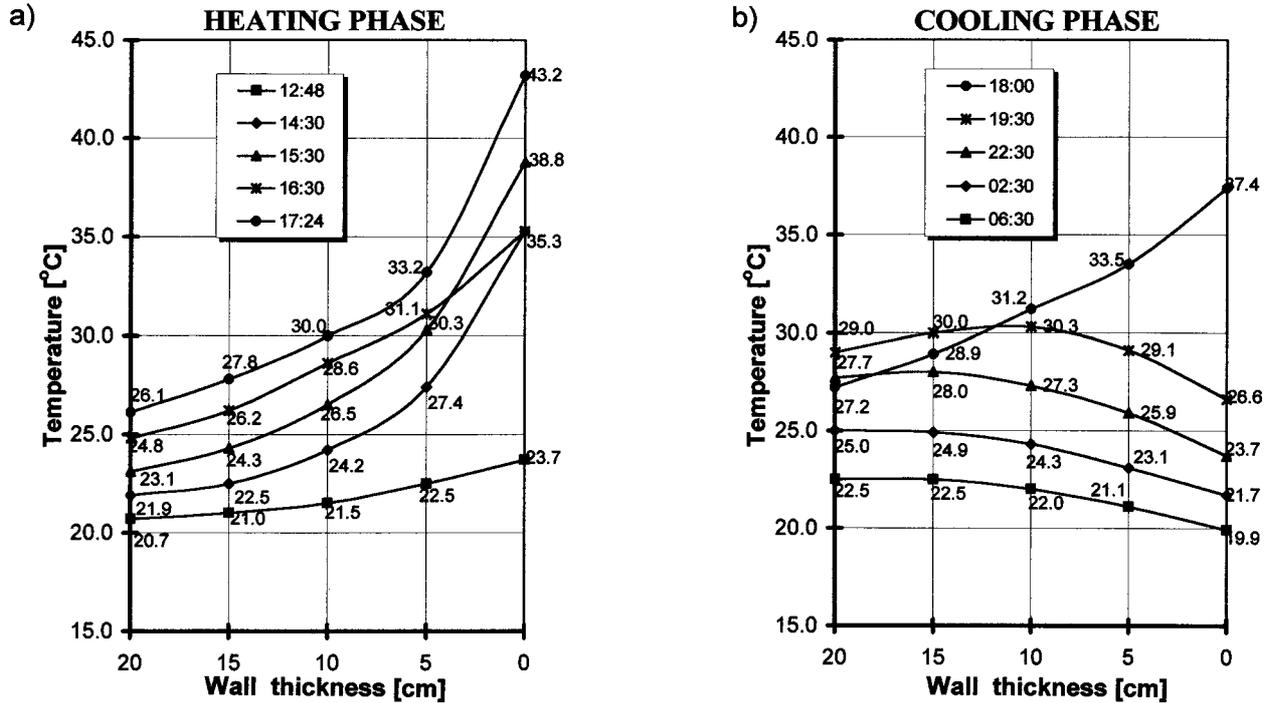
Fig. 1. Short time temperature changes across the concrete wall thickness of grain silo bin during heating and cooling of silo wall induced by daily temperature variations (Łapko and Prusiel, 1998).
