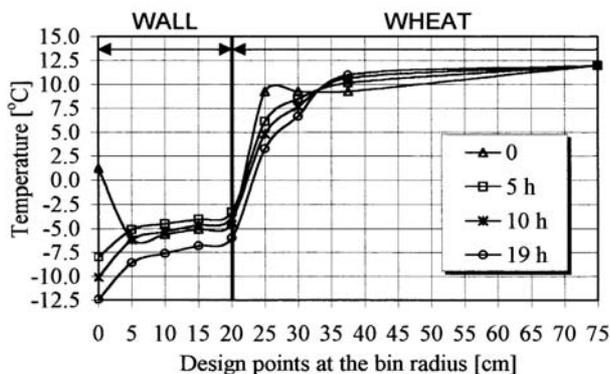
Fig. 3. Temperature changes predicted numerically along the silo bin radius during one day long phase of dropping winter temperature (Łapko and Prusiel, 2003).
