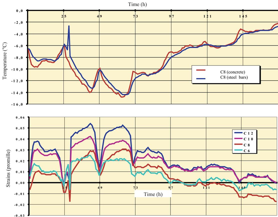
**Fig. 4.** Selected diagrams of silo wall temperature registered in winter 2002/2003 during 7 day period of monitoring (Łapko and Kołłątaj, 2003) – concrete silo for grain ‘in situ’.
