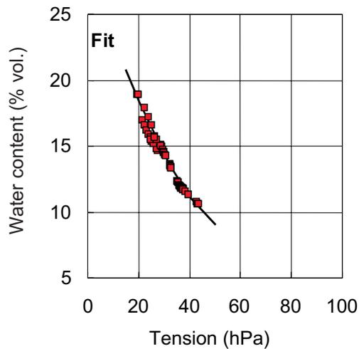
Fig. 4. Water retention curve, measured values and fit.
