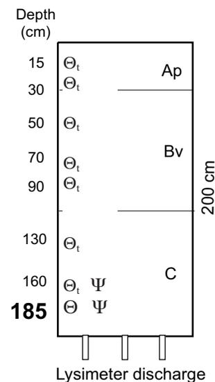
**Fig. 1.** Lysimeter construction,  $\Theta$  - TDR recording,  $\Theta_t$  - TDR probe for temporary measurements,  $\Psi$  - tension recording.
