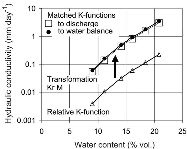
Fig. 5. Unsaturated hydraulic conductivity functions, relative and matched (effective) functions.
