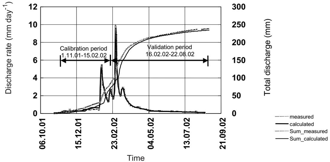
**Fig. 6.** Lysimeter discharge and deep seepage calculations, calibration to the discharge between 1st November, 2001 and 15th February, 2002.
