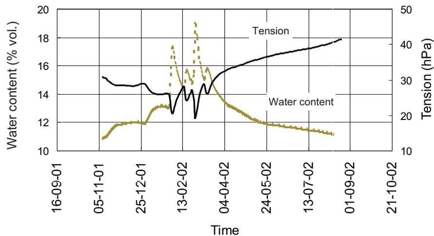
Fig. 2. Tension and water content dynamics, 185 cm depth (total period).
