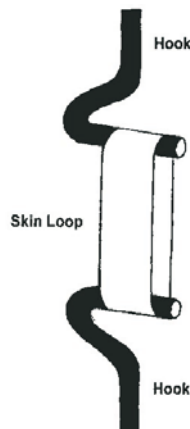
Fig. 2. Tomato skin ready for tension test.
