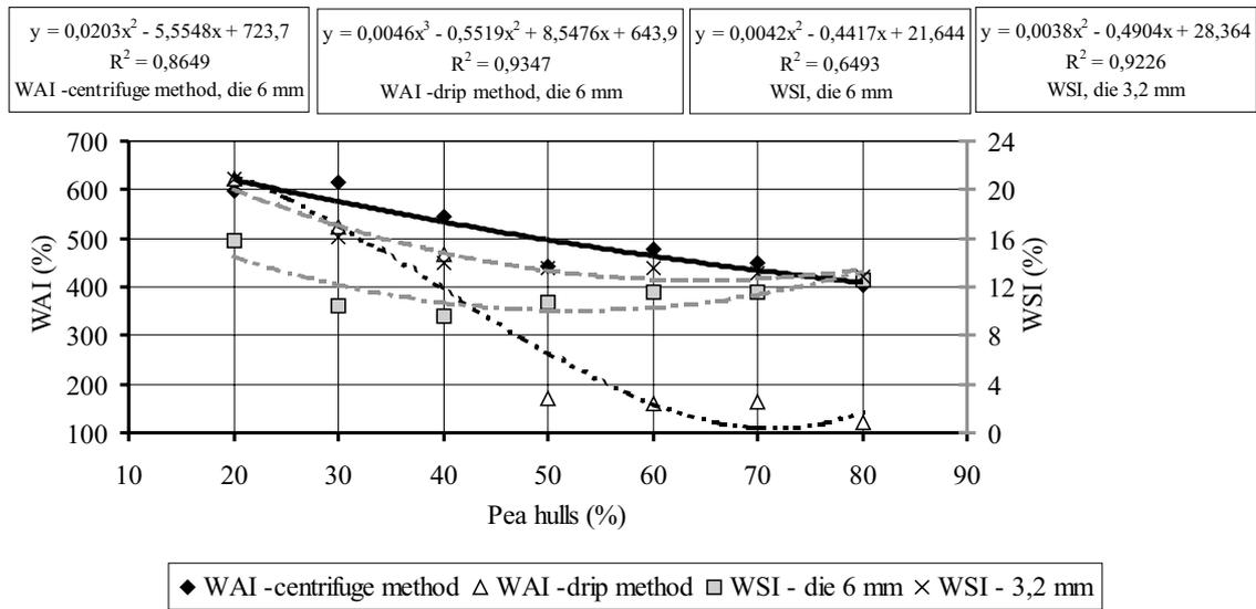
Fig. 4. Influence of the addition of pea hulls on the water absorption index (WAI) and the water solubility index of the extrudate (die diameter – 6 mm, moisture – 14%, temperature – 200°C, die diameter – 3.2 mm, moisture – 17%, temperature – 200°C).
