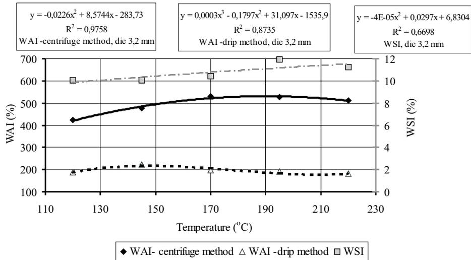
**Fig. 6.** Influence of barrel temperature on the water absorption index of the extrudate (WAI) and the water solubility index of the extrudate (WSI) (die diameter – 3.2 mm, moisture – 17%, rate of pea hulls – 40%).
