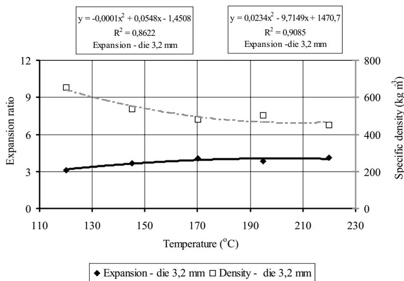
**Fig. 3.** Influence of the barrel temperature on the radial expansion of the extrudate and the specific density (die diameter – 3.2 mm, moisture – 17%, rate of pea hulls – 40%).
