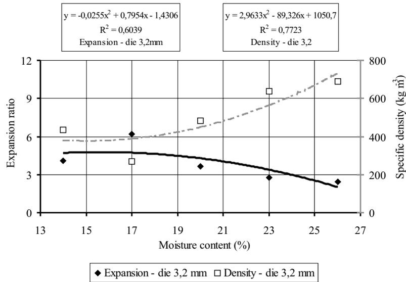
**Fig. 2.** Influence of the moisture of the raw material on the radial expansion of the extrudate and the specific density (die diameter – 3.2 mm, temperature – 200 C, rate of pea hulls – 40%).
