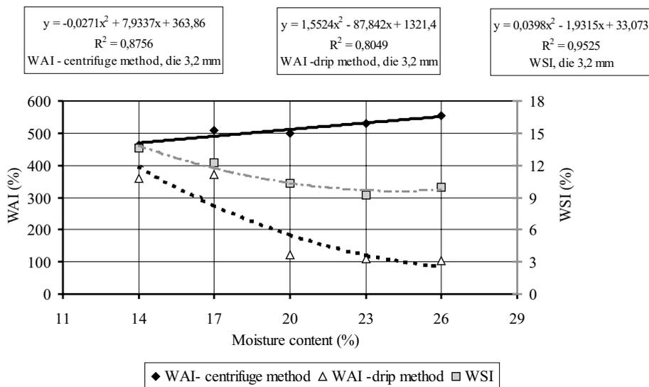
Fig. 5. Influence of the moisture content of the raw material on the water absorption index (WAI) and water solubility index (WSI) of the extrudate (die diameter – 3.2 mm, moisture – 17%, temperature – 200°C, rate of pea hulls – 40%).
