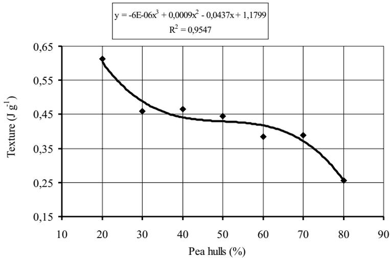
**Fig. 7.** Influence of the addition of pea hulls on the texture of the extrudate (die diameter – 6 mm, moisture – 14%, temperature – 200°C).
