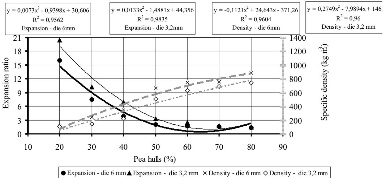
**Fig. 1.** Influence of the addition of pea hulls on the radial expansion of the extrudate and the specific density (die diameter 3.2 and 6 mm, moisture, respectively 17 and 14%, temperature – 200°C).
