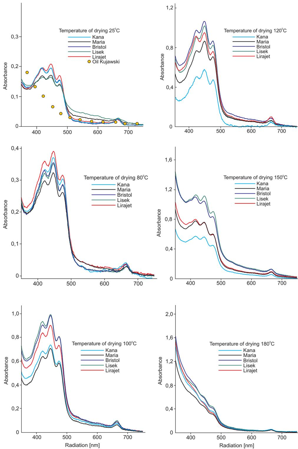
**Fig. 1.** Examples of absorption spectra recorded in the range of 350–750 nm from oil samples dissolved in acetone. In order to be measured, the oil samples were diluted 5–10 times. Different panels correspond to different drying temperatures (25–180°C), indicated.
