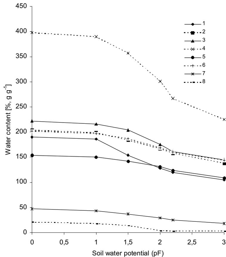
**Fig. 1.** Water retention curves for investigated soil samples (Nos 1–8), (water content in mass units (g g<sup>-1</sup>)).
