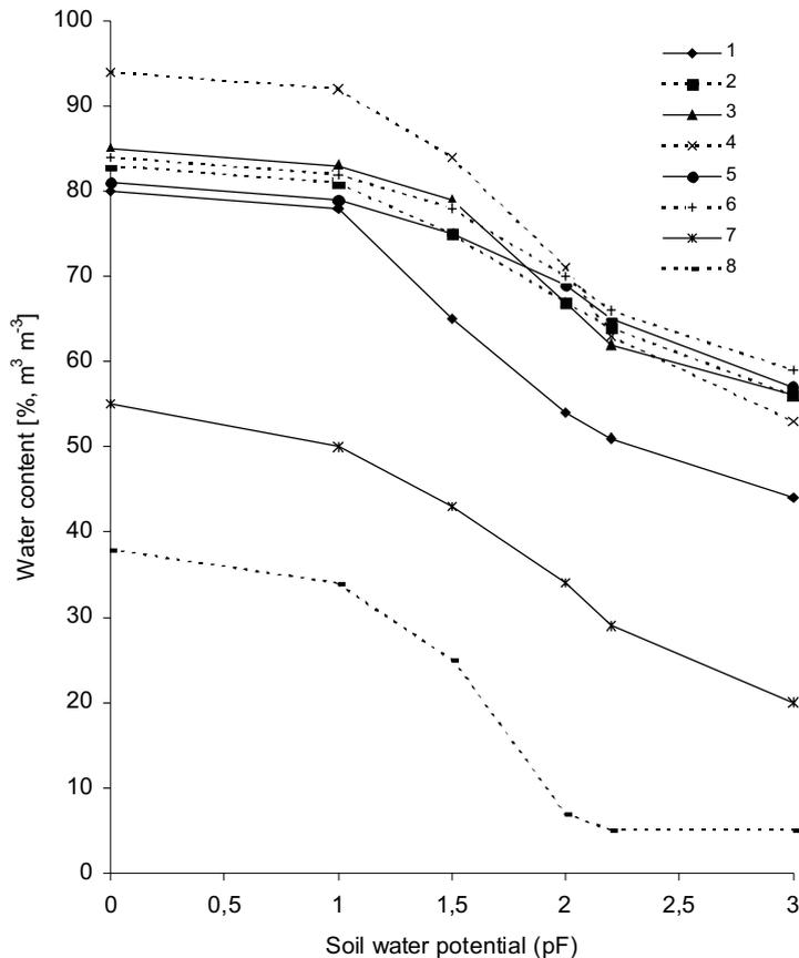
Fig. 2. Water retention curves for investigated soil samples (Nos 1–8) (water content in volume units ( $\text{m}^3 \text{m}^{-3}$ )).
