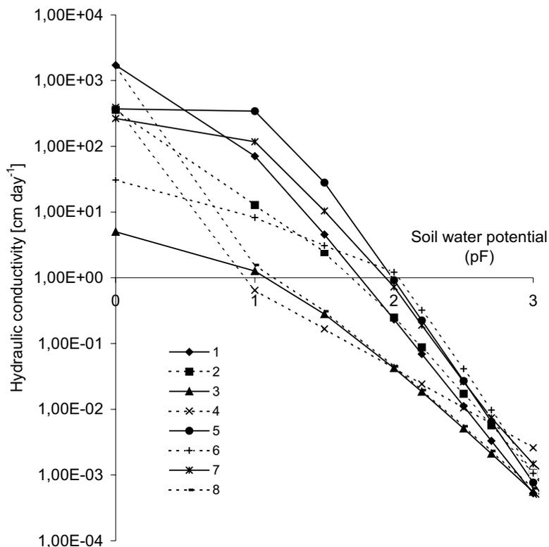
Fig. 3. Hydraulic conductivity at chosen soil water potentials for investigated soil samples (Nos 1–8).
