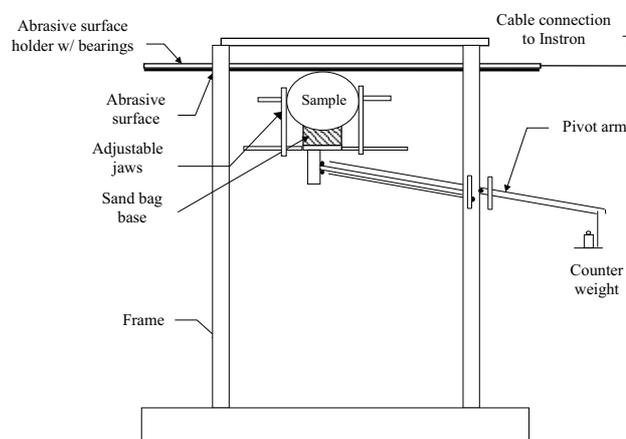
**Fig. 1.** Friction test device.
