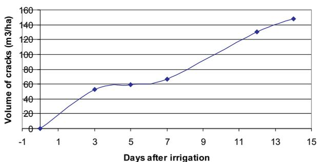
**Fig. 4.** Volume of cracks developed on the 3rd, 5th, 7th, 12th and 14th day after irrigation.
