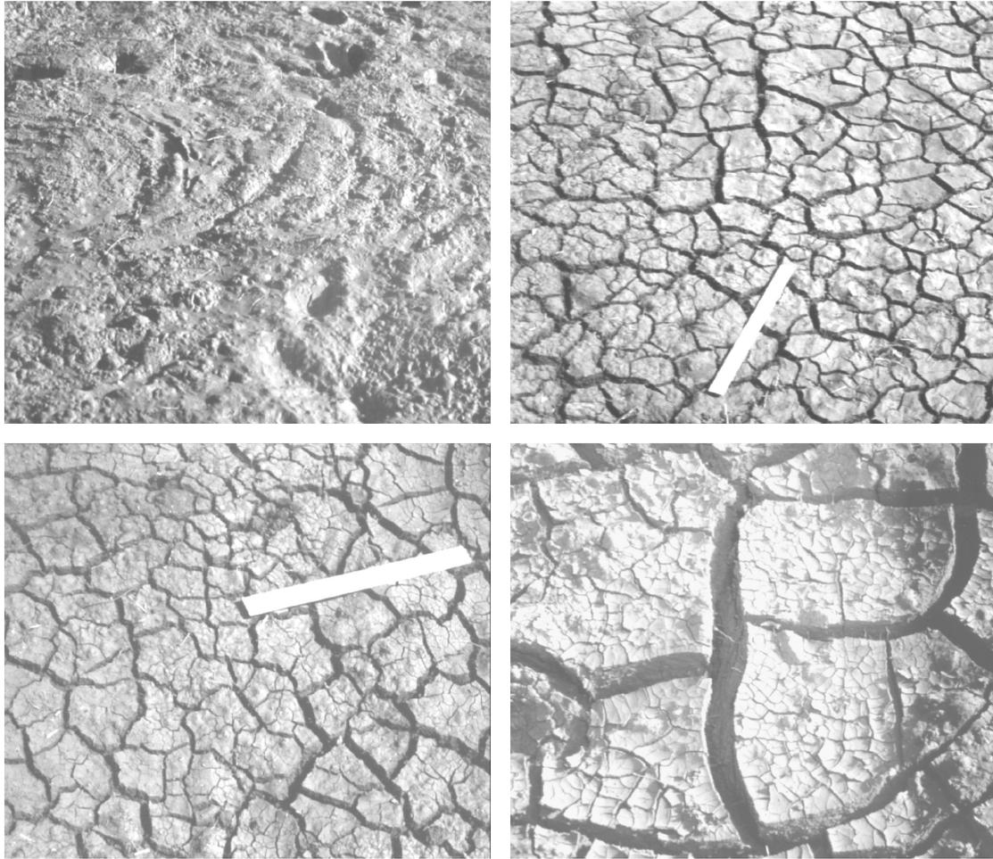
**Fig. 3.** Cracking patterns between the first and second irrigation treatments (no crop condition); day 1 (top left), day 3 (top right), day 7 (bottom left), day 12 (bottom right).
