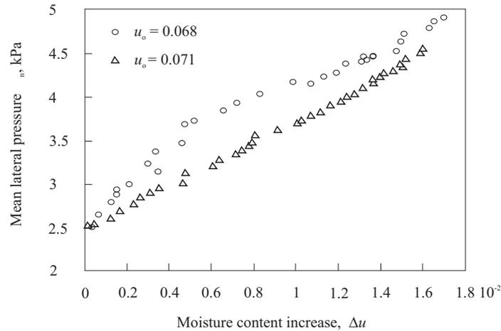
Fig. 5. Mean lateral pressure  $\sigma_n$  on the silo wall as influenced by the moisture content increase.
