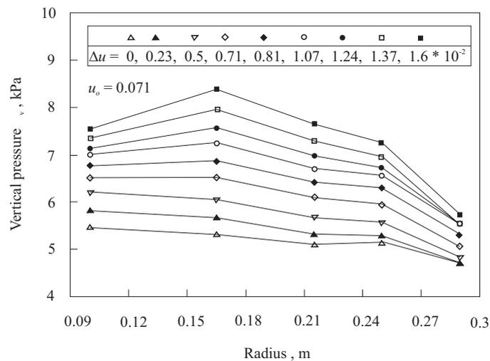
Fig. 4. Radial distribution of vertical pressure  $\sigma_v$  on the silo bottom as influenced by the moisture content increase.
