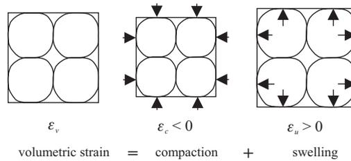
Fig. 1. Illustration of volumetric strain resulting from compaction by confining pressure and kernel swelling.
