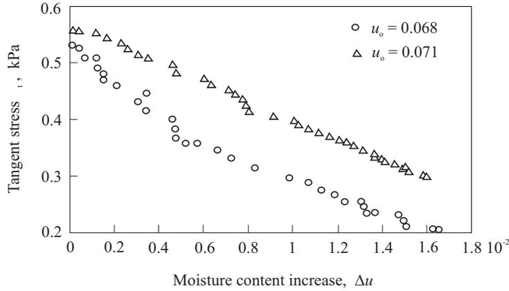
Fig. 6. Tangent pressure  $\sigma_t$  on the silo wall as influenced by the moisture content increase.
