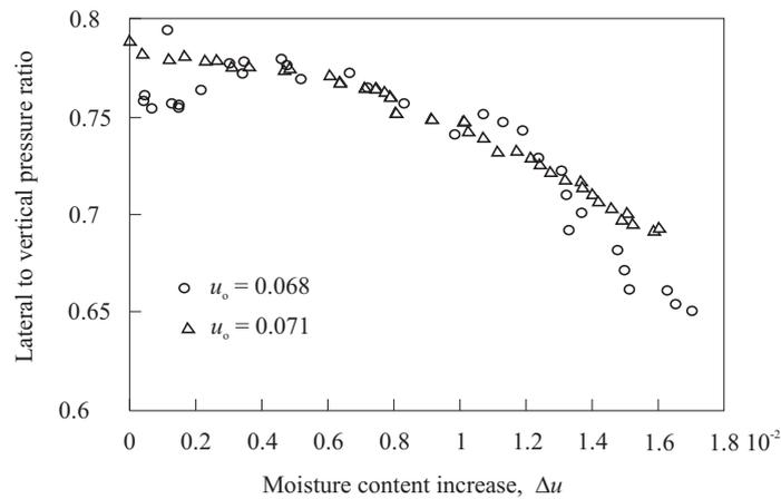
Fig. 7. Lateral to vertical pressure ratio as influenced by the moisture content increase.
