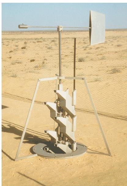
**Photo 1.** Sediment catcher with a vertical array of sediment traps.
